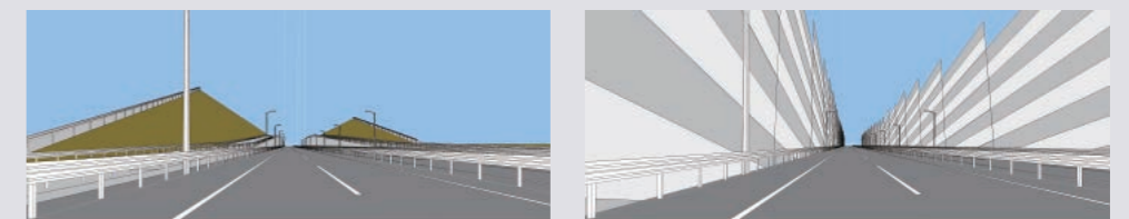
A simulation of the longitudinal gradient illusion (right) placed between the Anagawa Higashi Interchange and the Kaizuka Interchanges on Tokyo-bound Keiyo Road; Sidewalls that depict the tilted lateral stripe were placed to create the illusion. The road incline appears steeper when compared with the road side with no walls (left).
