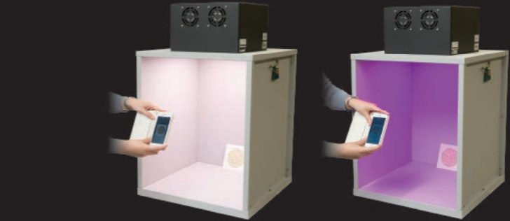
By making supplemental light of appropriate spectral distribution shine on objects, people with congenital color deficiency will be able to distinguish the color of those objects.
